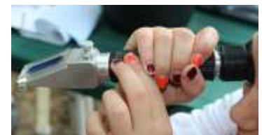
Testing parameters include salinity, measured with the refractometer shown at right.
